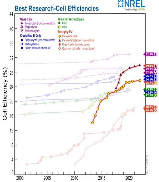
Efficiency records for perovskite PV cells compared to other PV technologies, with current records of 25.7% for single junction perovskite devices and 29.8% for tandem perovskite-silicon devices (as of January 26, 2022).
